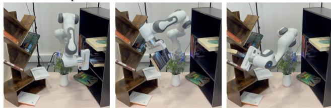
(c) Our policy has not been trained on this bookcase, yet it is able to insert the book into the correct location.
